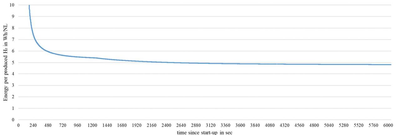
Figure 6 - Energy demand per produced hydrogen considering the starting energy of an AEMEL.
